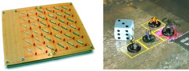
Figure 4: A custom game board sensing magnetic fields (left) and a touch display with camera recognition (right).
