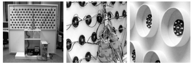
Figure 4. From left to right: 1) Rear view with control components 2) Wiring and transponders for each cell 3) Cells with LED clusters
