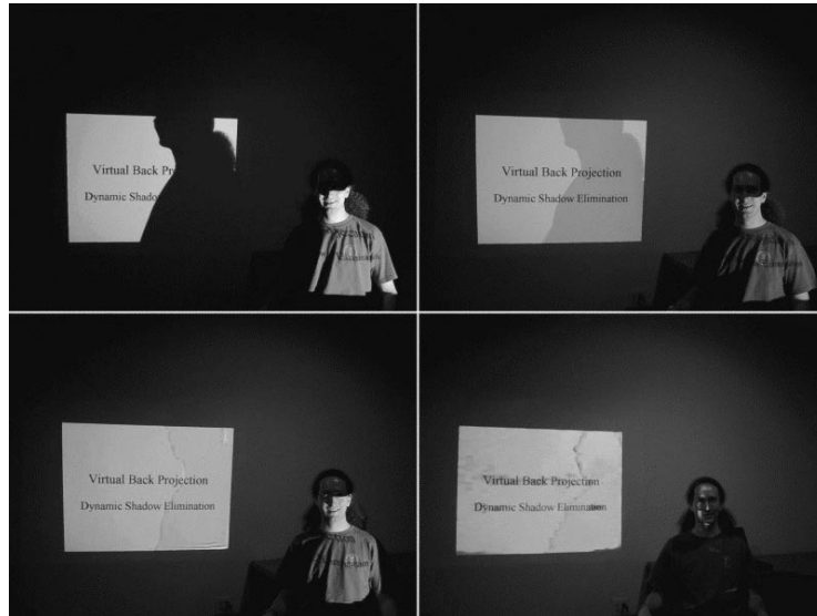
Fig. 1. Virtual Rear Projection: Single projector (top left). Dual redundant projectors (top right), with dynamic compensation (bottom left) and occluder light suppression (bottom right). A video and more detailed figures are available at: http://www.cc.gatech.edu/~summetj/research.html
