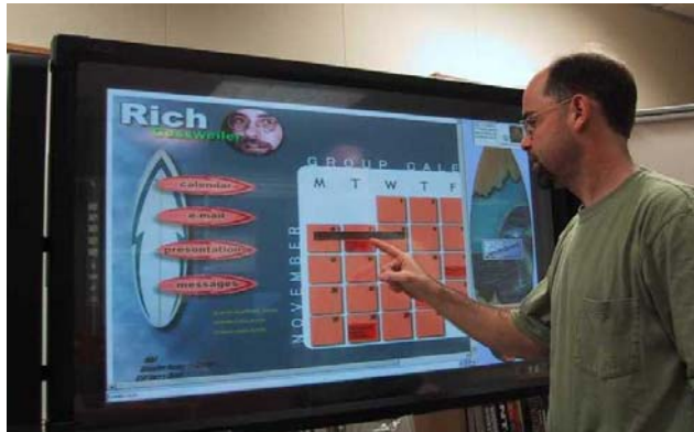
Fig. 1. The BlueBoard is a Large Scale Information Appliance offering fast access to personal information with tools for collaboration and small groups of people working side-by-side. The display has a touch screen overlay and a badge reader on the right corner for person identification. Network access is assumed.
