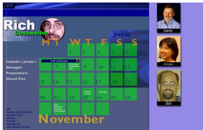
Fig. 2. A typical BlueBoard personal display. This kind of content is set up by each user as their "home content." Content displayed on the BlueBoard can be shared with another person by dragging the content (window, image, URL) to their p-con. Here, Rich is showing his home page calendar to Daniel and Alison.
